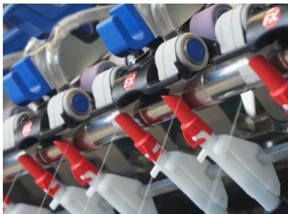
New suction tube with optimised bracket.
